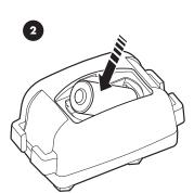
Insert the battery, ensuring that the + (plus) and – (minus) terminals are aligned correctly.
